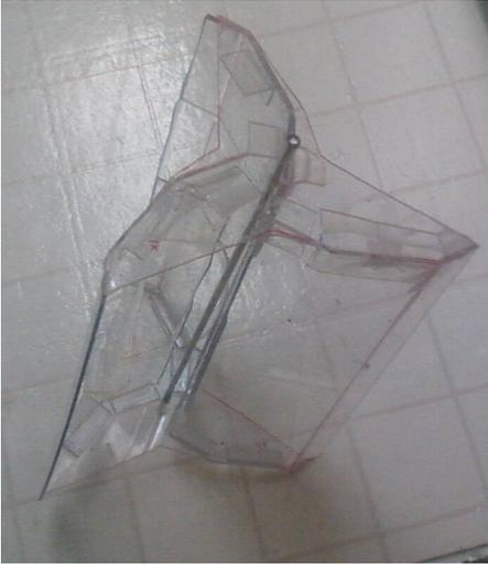
This turbine design is nearly immune to the effects of turbulent air which can destroy the efficiency of most other designs. This feature makes it feasible for use directly mounted on short fence posts rather than requiring tall poles.
