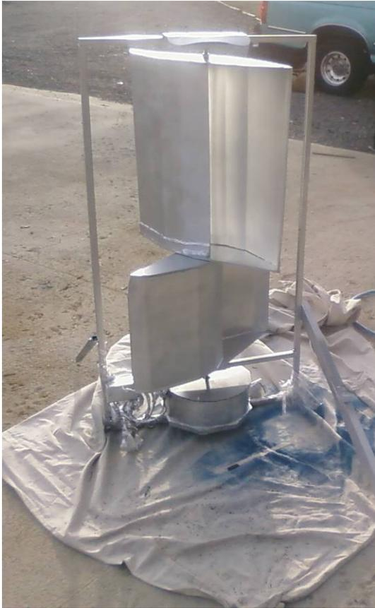
Completed 165 watt @ 28 MPH winds designed and build by Joseph Ellsworth Winter 2008. Includes PMG alternator capable of reaching 48 V charging at 80 RPM or 12 MPH winds.
